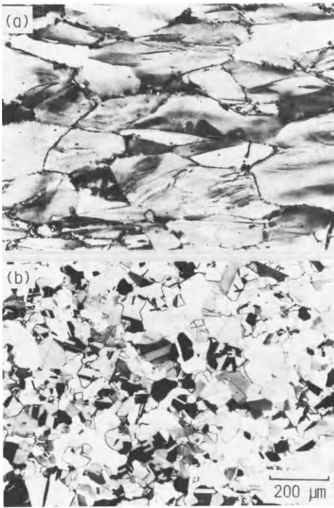
Figure 2.15 Optical micrographs showing the static recrystallization occurring during isothermal holding of heavily work-hardened \gamma in Fe–31 Ni–0.3 C austenitic alloy: (a) work-hardened \gamma (deformed at 900° C, \dot{\epsilon} = 3/s , \epsilon = 1.0 ); (b) static recrystallized \gamma (isothermally held at 900° C for 50 s of structure (a))
